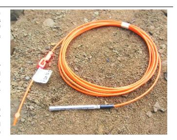
One of its ends is ultrasonically sealed and the other end is assembled to the Delay Detonator. The color of the Fanel Hose UV allows to identify Fanel UV delay time scale, so: For the short period the Fanel Hose UV is orange (MS); for the long period the Fanel Hose UV is yellow (LP).
